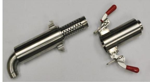
**Figure 3: Insert the Filter Paper into the Perforated Cylinder**
