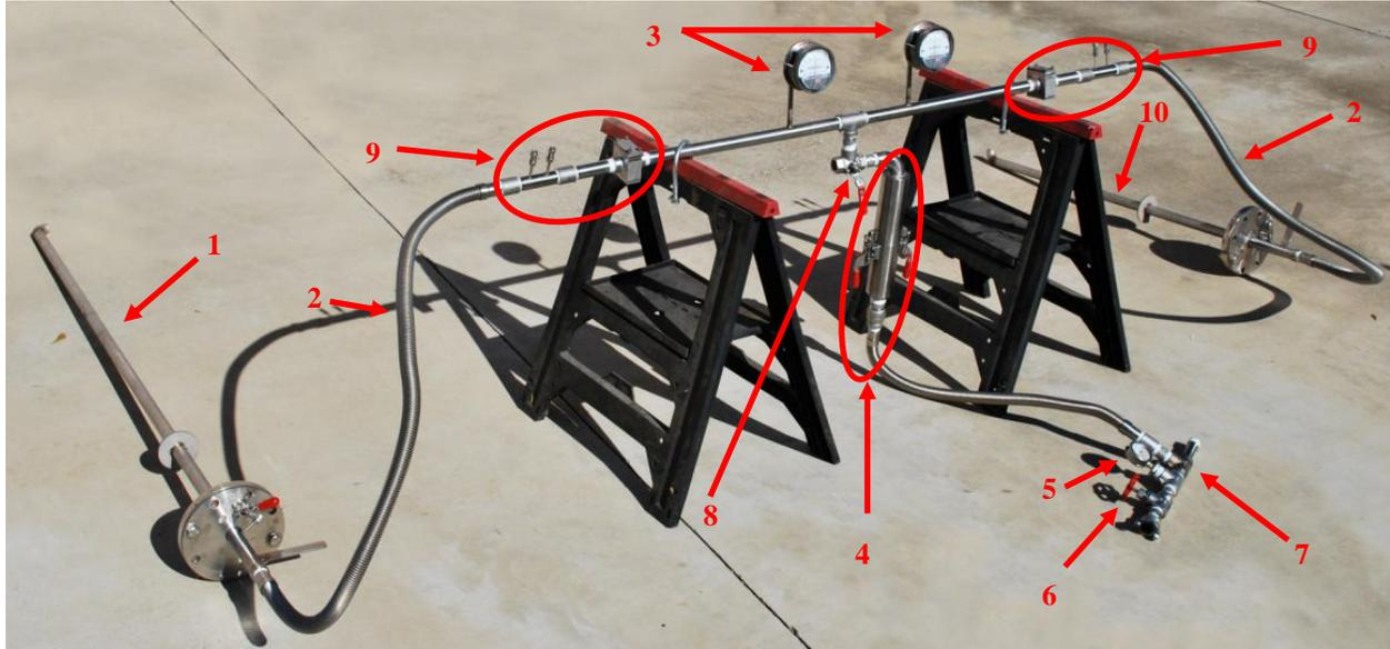
Figure 1: Fully Assembled Permanently Mounted Volumetric Flyash Sampler
