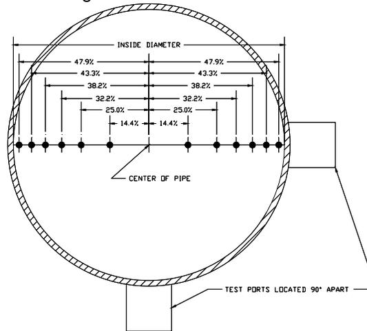
NOTE: EACH PERCENTAGE IS MULTIPLIED BY THE INSIDE DIAMETER OF THE PIPE TO SHOW THE SAMPLING POINT.
