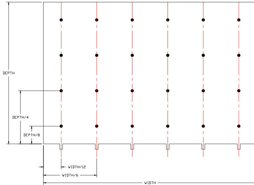
**NOTE:** IT IS IMPORTANT TO HAVE A SUFFICIENT NUMBER OF SAMPLING POINTS FOR REPRESENTATIVE MEASUREMENTS. THE DIMENSIONS ON THE SKETCH ABOVE MAY VARY DEPENDING ON THE NUMBER OF TEST TAPS REQUIRED DUE TO SIZE OF DUCT BEING TESTED.
