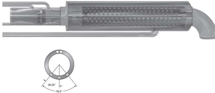
Figure 3 - Flue inserted High Volume Flyash Sampler
